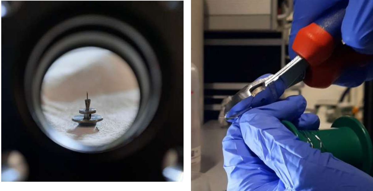
Figure 79: Left: Tip in the tipholder , Right: How we cut the tip.
