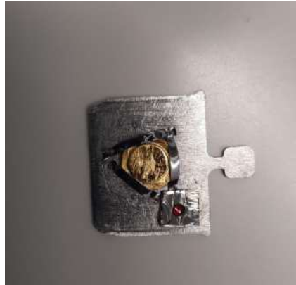
Figure 40: Sampleholder with gold crystal fixed with spot yielded Ta foil and AuNPs applied on HOPG fixed with silver glue.
