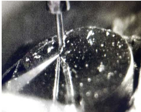
Figure 44: Alignment of the fibre LFM1F-1. We see the gold crystal, the tip in the middle and its reflection in the sample. The bright line coming from the bottom left pointing to the tip is the fibre tip.
