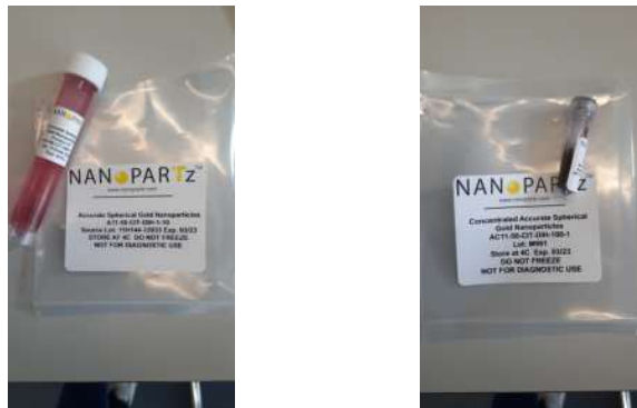
Figure 31: Left: "Accurate Spherical Gold Nanoparticles" - 50 nm, Capping Agent Citrate, Buffer DIH, OD 1, 10mL, Right: "Accurate Concentrated Spherical Gold Nanoparticles" - 50 nm, Capping Agent Citrate, Buffer DIH, OD 100, 1 mL
