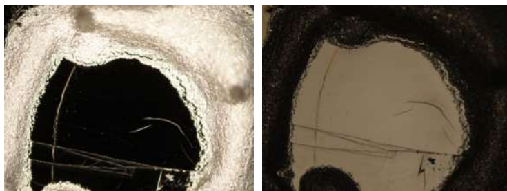
Figure 91: With silver glue we made small circles on HOPG and performed dropcast of 1 \mu L in each circle.
