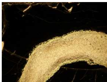
Figure 92: With silver glue we made small circles on HOPG and performed dropcast of 1 \mu\text{L} in each circle. Additionally we heated the sample afterwards with 300° for 20 min.
