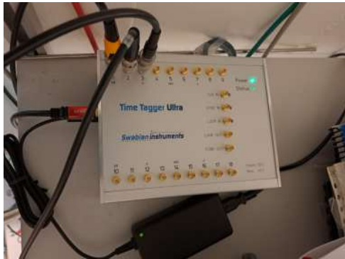
Figure 47: The timetagger of Swabian instruments. Output 2 was connected to the Photon counter and Output 3 was connected to the STM controller trigger port (see Figure 48).
