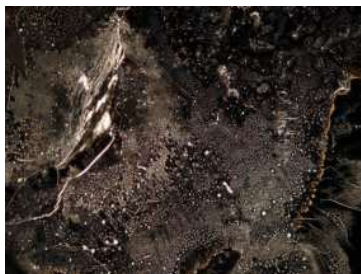
Figure 85: Dropcasted gold nanoparticle solution (OD1, air, room temperature) onto HOPG taken with the light microscope BX41M. On the left we listed the used objective with their corresponding magnification. In the 100x magnitude we see that liquid is surrounding the particle clusters.
