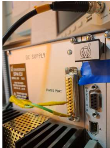
Figure 48: Trigger port of the STM control electronics that we connected to the time-tagger. The scan produces a line trigger for every scan line, enabling us to produce a spatially dependent photon map. To connect the pins we used the information provided in the SCALA pro manual (see Figures 72 and 73).
