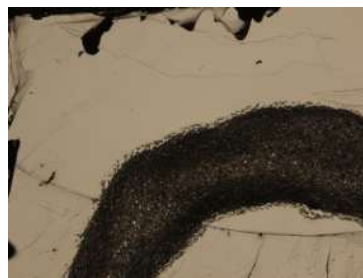
Figure 92: With silver glue we made small circles on HOPG and performed dropcast of 1 \mu\text{L} in each circle. Additionally we heated the sample afterwards with 300° for 20 min.
