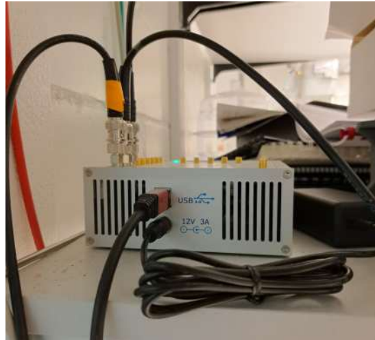
Figure 47: The timetagger of Swabian instruments. Output 2 was connected to the Photon counter and Output 3 was connected to the STM controller trigger port (see Figure 48).
