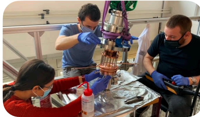
Installation Cold Head Cry-Tower
