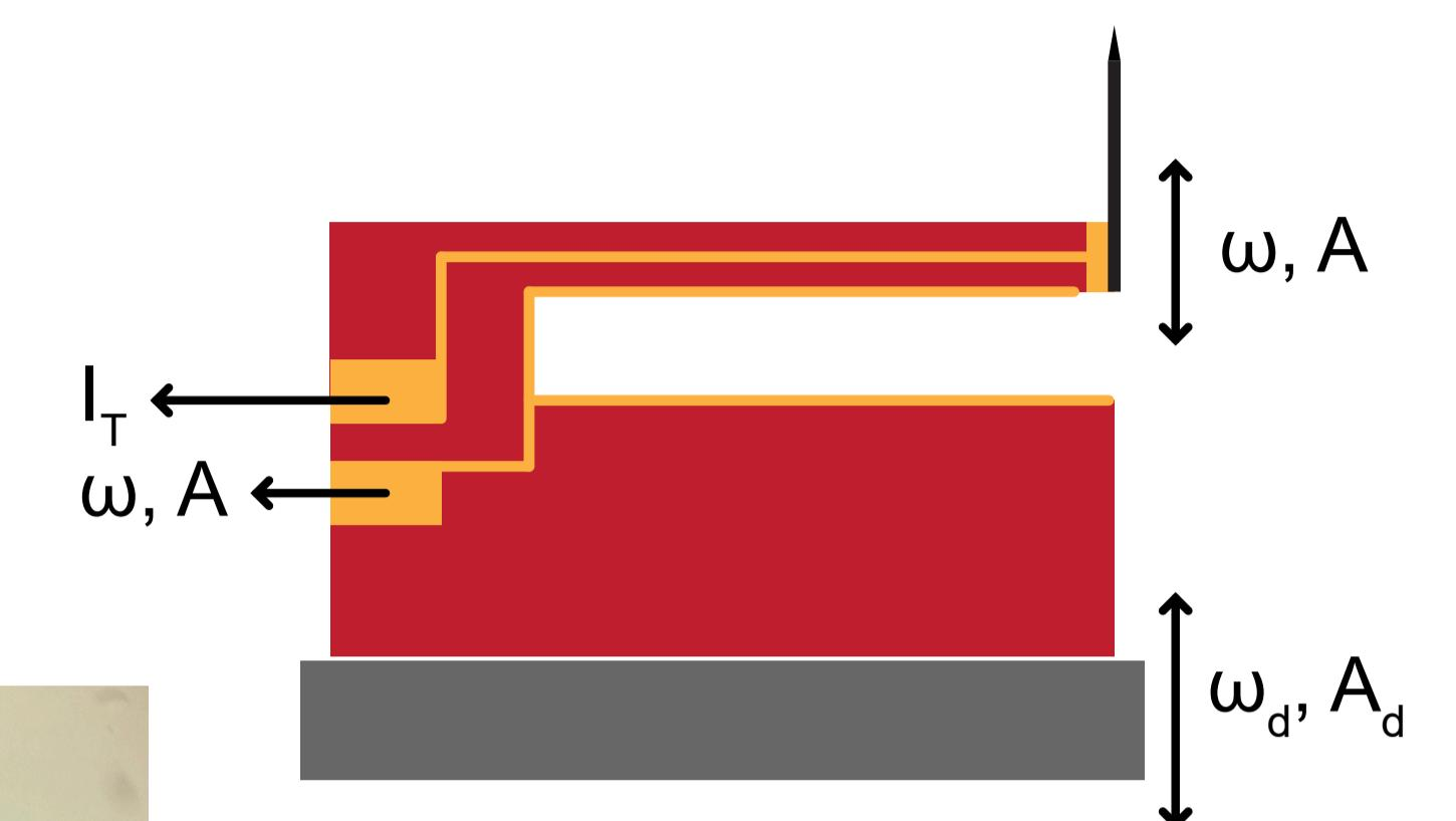
$$\begin{aligned} A &\approx 20 - 100 \text{ pm} \\ \omega &\approx 30\,000 \text{ Hz} \\ Q &\approx 40\,000 - 100\,000 \end{aligned}$$
