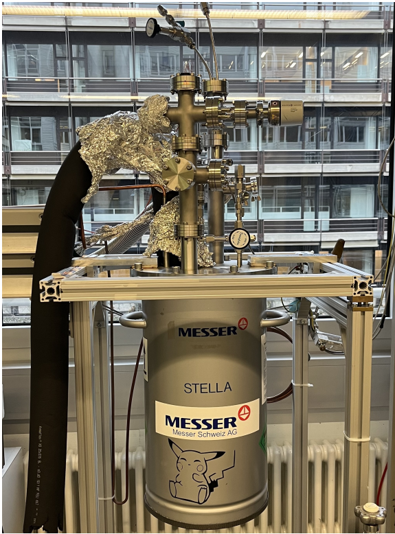
Figure 14: The external setup of LArS showing the cooling system and the vessel.
