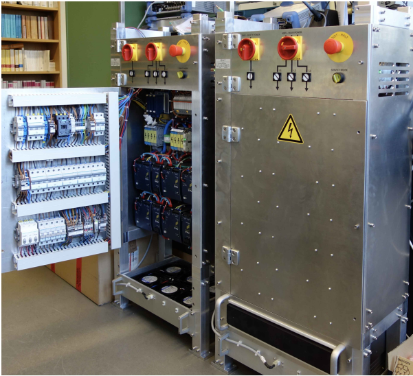
FIG. 6.2 – Two safety and power cabinets under 24/7 testing before installation into the camera.
