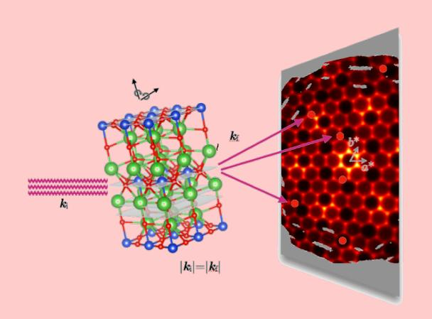
In diffraction experiments the incoming x-ray beam and the scattered waves give rise to a complex constructive and destructive interference effect. The resulting diffraction pattern depends on the relative arrangement of the constituents of the crystal lattice.
