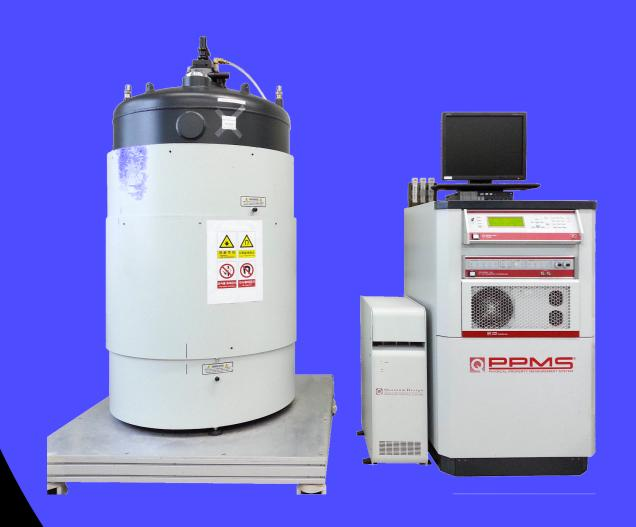
A PPMS allows for systematic measurements of macroscopic physical properties such as the resistivity  $\rho$ , magnetization  $\mathbf{M}$  or the heat capacity  $\chi$ . These observables can be measured as functions of the temperature T, an applied voltage or mechanic strain or pressure.
