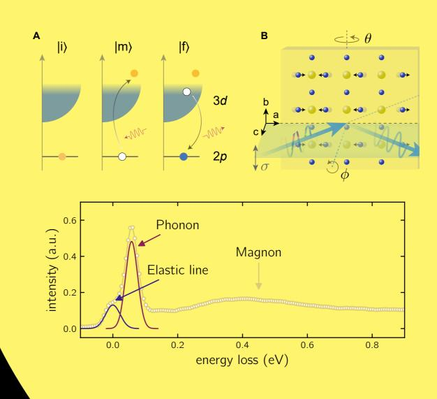
In a RIXS process, photons transfer energy and momentum to the sample and leave behind excitations in lattice, charge, spin, and orbital degrees of freedom.
