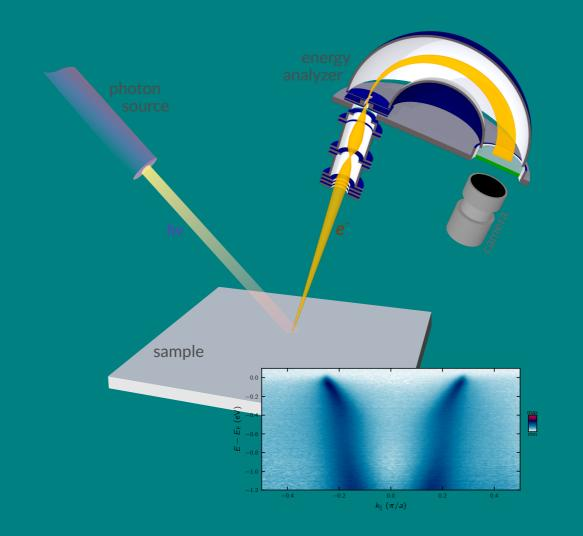
ARPES is a photon in, electron out experiment based on the photoelectric effect. The ejected electrons are sorted according to their momentum and energy. This allows us to directly probe the electronic dispersions inside a sample.
