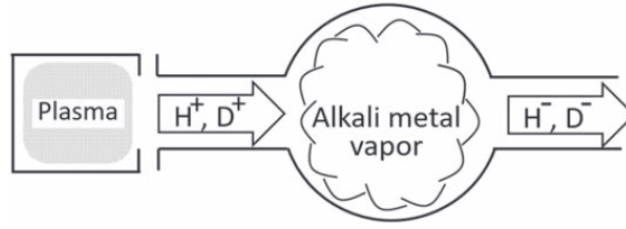
Figure 2.1: Schematic illustration of a double charge exchange source. The picture is taken from [6].
