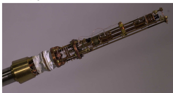
Figure 10.6: New heat-capacity probe with suspended measuring cell and AC-coils.
