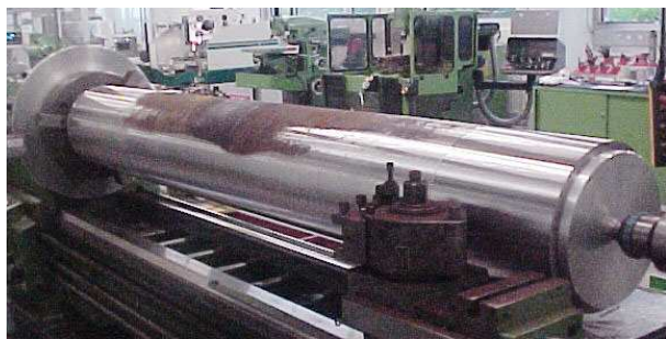
Cylinder used for the construction of the CMS pixel detector supply tubes.
