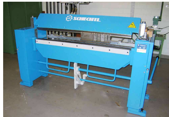
The new folding machine installed in the workshop.
