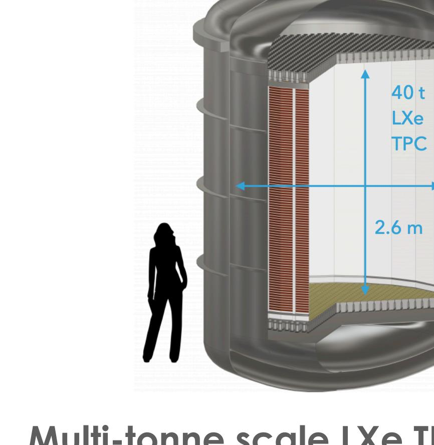
Multi-tonne scale LXe TPCs require R&D test platforms
