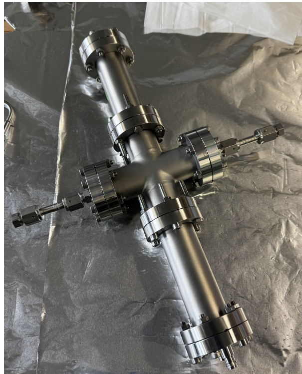
Figure 32: Photograph of the fully assembled cross detector before installation into the experimental setup. The two opposing PMTs are mounted along one detector axis, while the tube along the other axis forms the gas-flow path through the active scintillation region.
