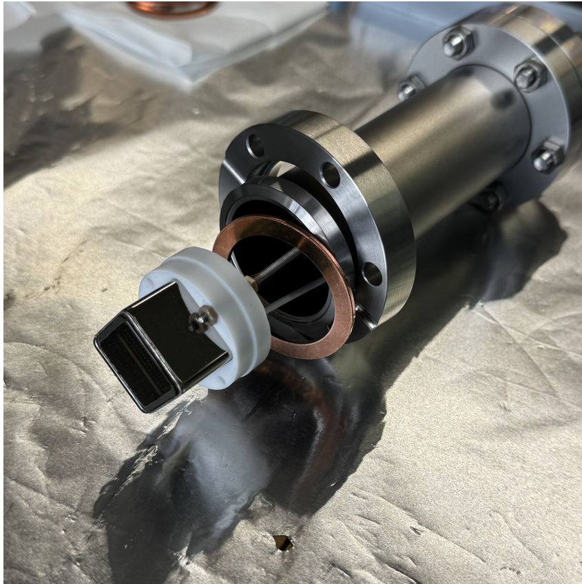
Figure 30: One of the selected R8520 photomultiplier tubes mounted in its PTFE holder during assembly. The holder provides mechanical support and electrical insulation from the surrounding metal components.
