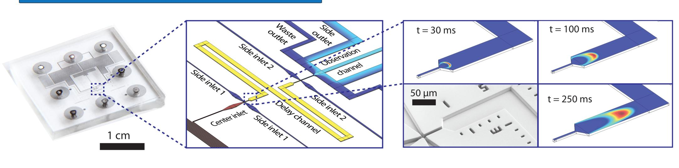
advantage of added microfluidic devices is that, due to the absence of turbulence, the full mechanics underlying these laminar flow systems can be calculated even for complex geometries with the help of finite-element methods. Experimentally determined flow velocities can therefore be directly
