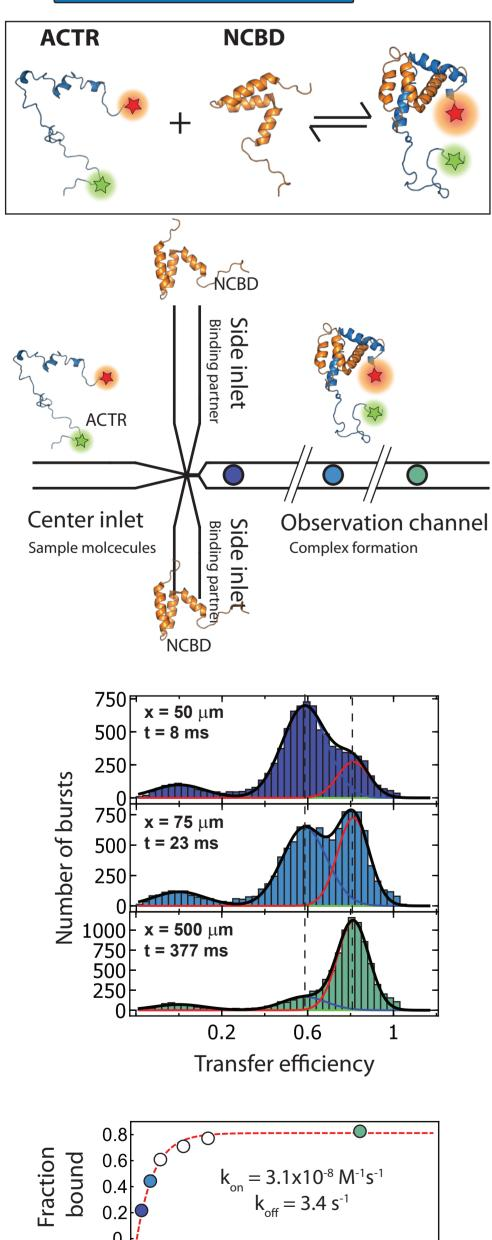
The microfluidic mixing device (1) can be used obtain netics timescales from milliseconds to minutes.
