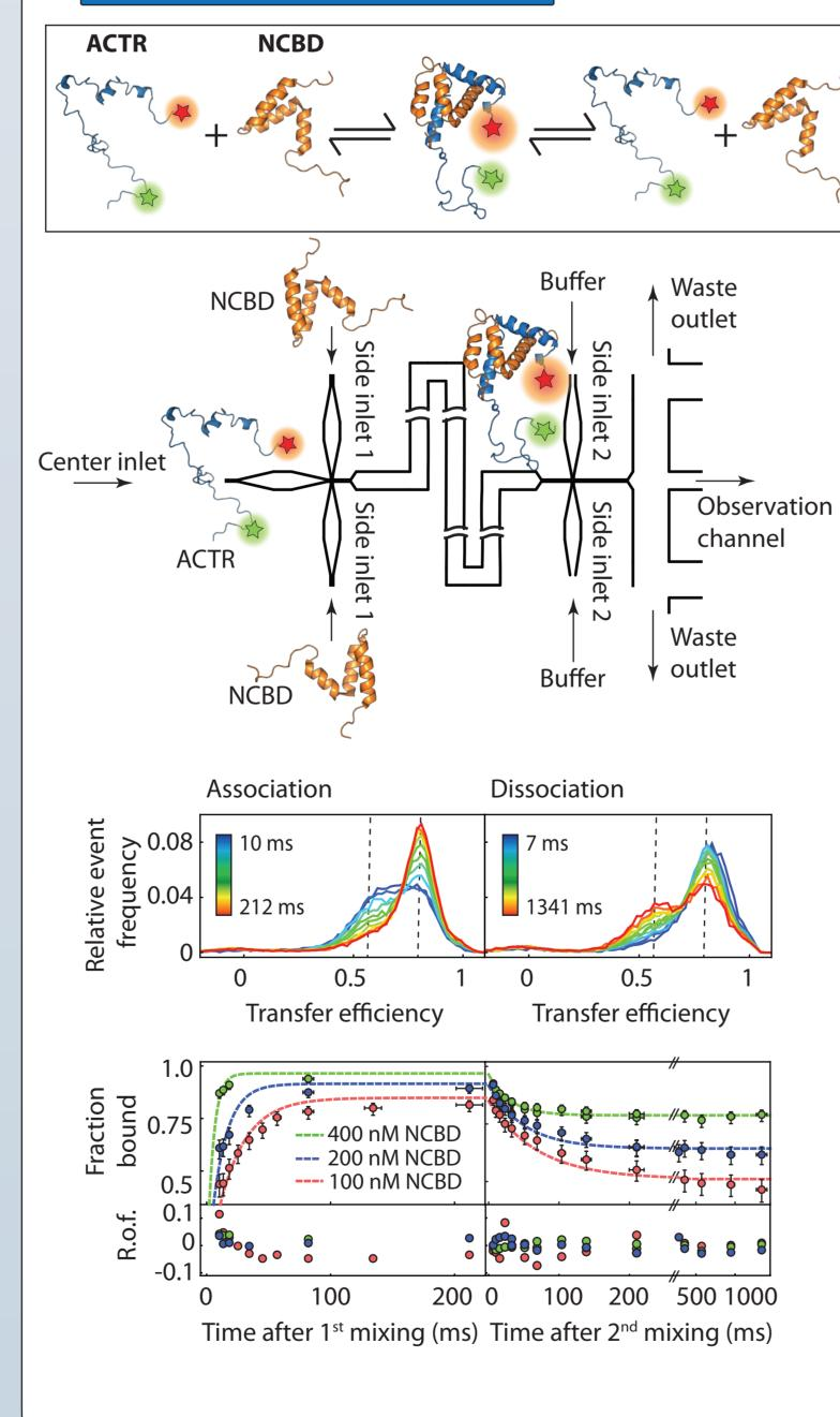
Recently, we extended microfluidic mixing also doubenable le-jump experiments (2). After a first mixing step, the sample molecules spend a defined time in a delay channel and can then be probed also after a second mixing step. This technique is particularly suited to investigate kinetic properties of transiintermediate species, but can also be used to study the association and dissociation of e.g. intrinsically disordered proteins, as shown here.
