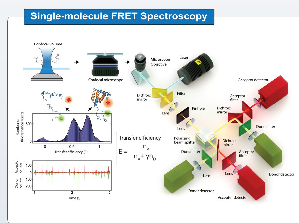
single-molecule Confocal FRET on freely diffusing fluore-The molecules: scence signal is first separated by polarization and then by wavelength into the detection channels corresponding to emission from donor and acceptor chromophores. By analyzing each of the fluorescence bursts, a histogram of transfer efficiencies can be calculated and different subpopulations exhibiting different transfer efficiencies can be distinguished.
