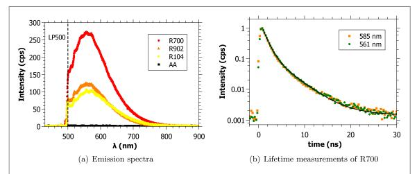
**Figure 5.** (a) Emission spectra of R700 (red dots), R902 (orange triangles), R104 (yellow diamonds) and AA (black squares) with  $\lambda_{\rm inc}=485$  nm using a long pass 500 nm filter and a laser power of  $P=50~\mu{\rm W}$ . (b) Lifetime measurements for two different incident wavelengths (585 nm (orange squares) and 561 nm (green dots)). The corresponding bi-exponential fit is shown as black line. The first exponent corresponds to the electronic setup response and can be ignored.
