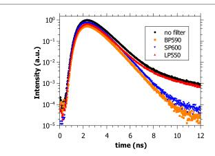
**Figure 4.** To F distribution of a R700 sample (L=0.83 mm) measured without filter (no filter), a bandpass filter around 590 nm (BP590), a shortpass filter 600 nm (SP600) and a longpass filter above 550 nm (LP550) with an incident wavelength  $\lambda_{\rm inc}=590$  nm. The red shifted photons show a long time tail, indicating a fluorescence while the blue shifted and non-shifted light behaves purely diffusively.
