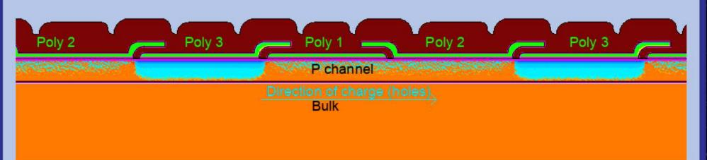
In addition, these CCDs use three-stage polysilicon gates, which minimizes the loss of charges generated by particles interacting in their bulk.
