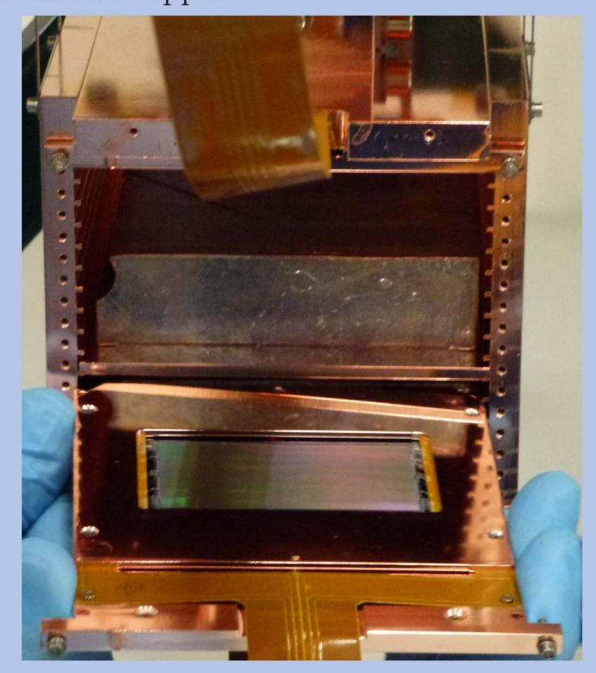
These large, thick CCDs have a huge advantage over other solid state detectors as the interface to electronics are far from the pixels and therefore each pixel generates very low leakage current (below  $9 \times 10^{-22} \,\mathrm{A\,cm^{-2}}$ ).
