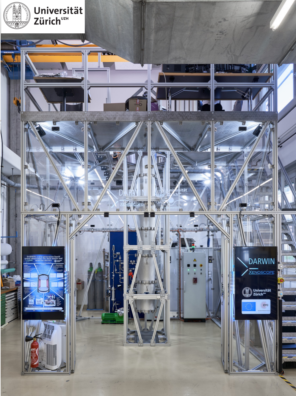
Test e^- drift over 2.6 m (purification, high-voltage)
