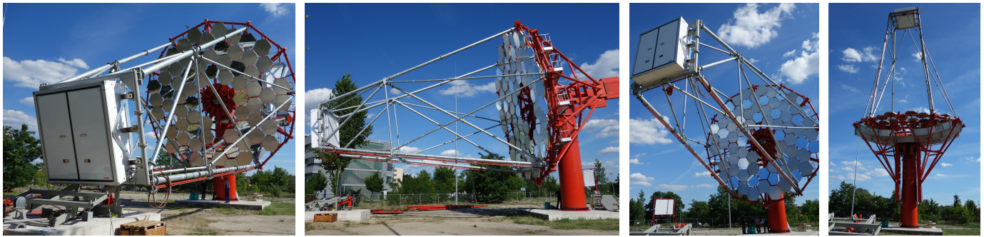
FIG. 6.2 – Rotating the telescope into the zenith position. The sledge, which can be moved with a winch, is visible below the camera body in the first picture. The camera lid is closed and the two installed detectors are read out for off-line study of possible light leaks and pick-up noise.
