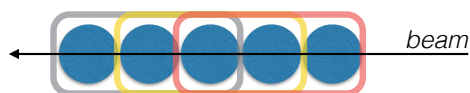
FIG. 7.6 – Principle of the efficiency measurement. For each fibre a cluster of three fibres is used (grey, yellow, red in this example) to specify the efficiency of the fibre in the middle of a cluster.
