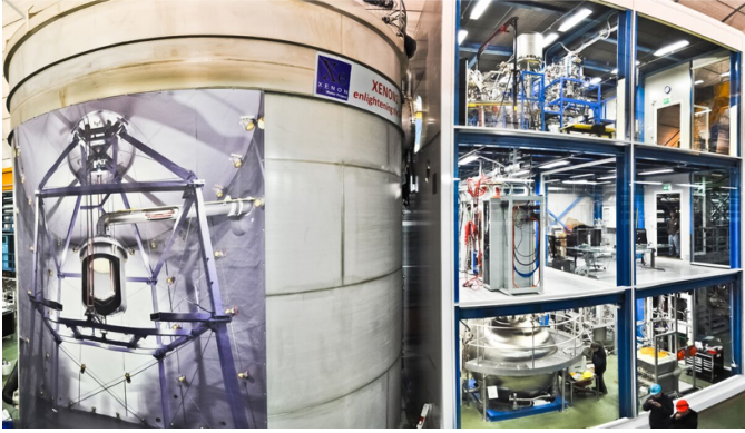
FIG. 4.3 – The XENON1T experiment in Hall B of LNGS. The water Cherenkov shield with a picture of the cryostat, its support structure and the pipe housing the cryogenic lines and cabling are seen on the left side. The infrastructure building, containing the LXe storage and purification systems, the krypton distillation column, the electronics and DAQ, as well as the cryogenic systems on the top level is seen on the right.
