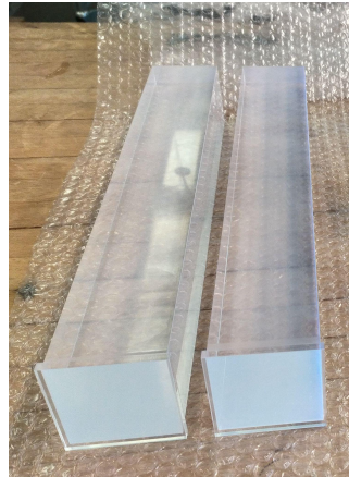
Figure 19: Two BC-412 plastic scintillators made of Polyvinyl Toluene(PVT) used for the muon detectors. Plastic scintillators have a low decay time of a few nanoseconds making them the choice for our setup where the detectors will be used for tagging muon events.
