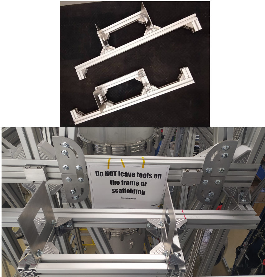
Figure 31: (top) Frame for the detectors assembled using aluminium profiles. (bottom) Frame of the detectors attached to the inner frame of the demonstrator. The cut outs in the two aluminium plates allow the muon detectors to be fixed properly.
