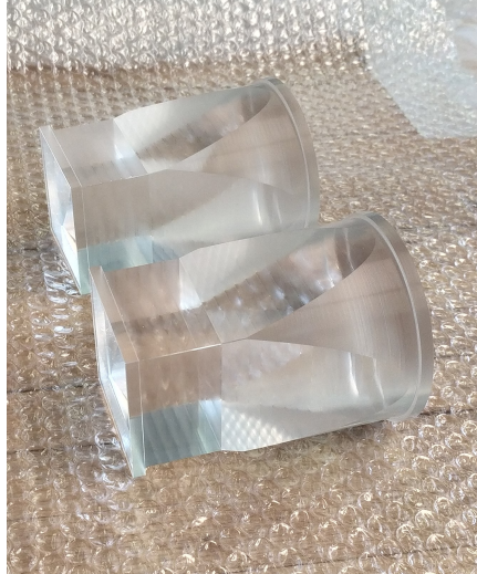
Figure 21: Lightguide fabricated by the mechanical workshop in the University of Zurich. It is made of acrylic material whose refractive index is 1.495. The lightguide is tapered at an angle of 11^\circ .
