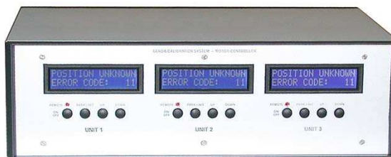
FIG. 18.7 – Motor control unit (front view).
