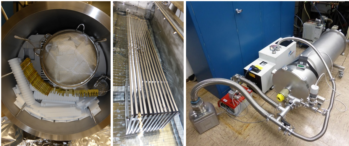
Figure 3.18: Left: The interior part of the vacuum transportation vessel for the PTFE, Torlon ® and PEEK ® parts. Centre: The PTFE reflector panels inside the ultrasonic bath at the University of Münster. Right: The transportation vessel connected to the gas system in order to evacuate it and to fill with pure nitrogen gas (6.0).
