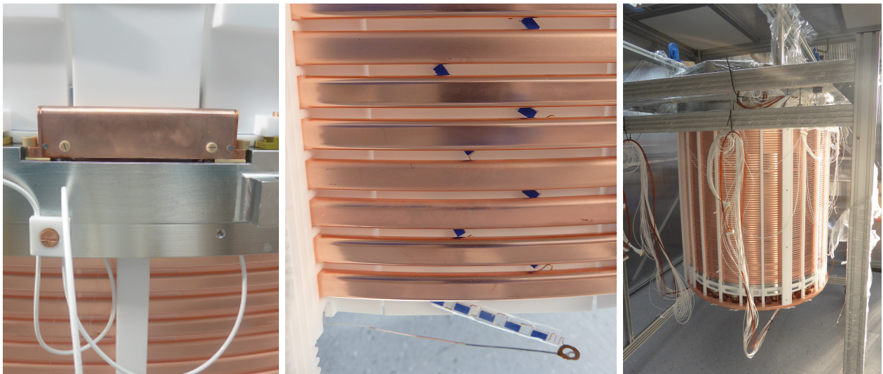
Figure 3.21: Left: The short levelmeter assembled to the top TPC ring. Centre: The resistor chain contact to the cathode. Right: The assembled TPC in the aboveground clean room attached to the support structure.
