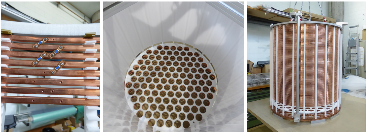
Figure 3.14: Left: The Kapton ® foils with the soldered resistors on top, screwed to the inside of the field shaping rings. Centre: The inside of the field cage enclosed by the PTFE reflector panels. The bottom PMT array copper plate and PTFE reflector were attached to the field cage. Right: The assembled field cage with the support structure.
