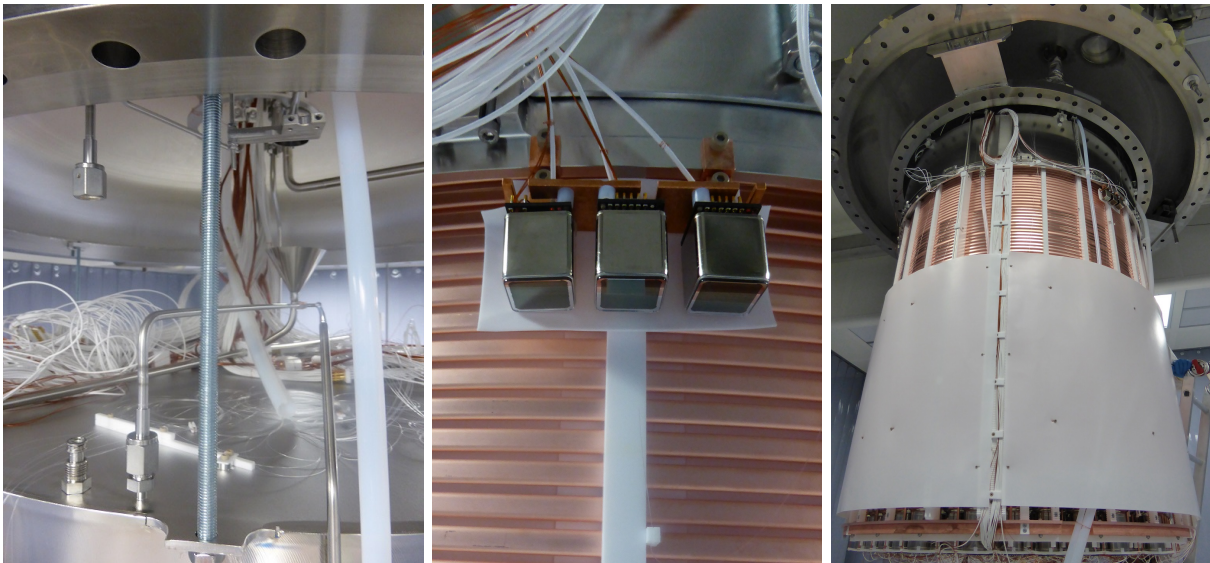
Figure 3.22: Left: The TPC in an intermediate position in order to perform all of the connections on top of the diving bell. Centre: Three out of the six installed ‘diagnostic’ PMTs. Right: The TPC in the final position before the cryostat closing with the attached PTFE high voltage sheet.
