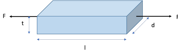
Figure 2.5: A thin film with dimensions l \times d \times t and tensile strain applied along the t \times d normal.
