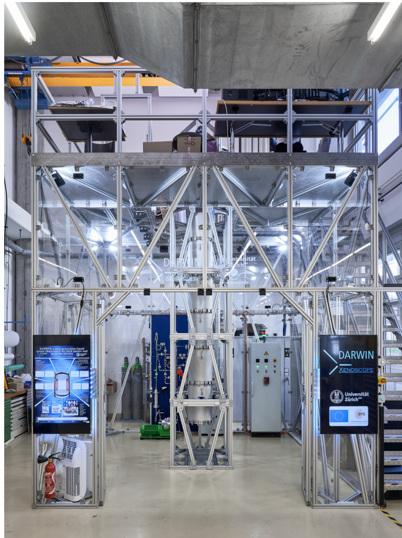
Test e^- drift over 2.6 m (purification, high-voltage): U. Zurich (G-floor Assembly Hall)
