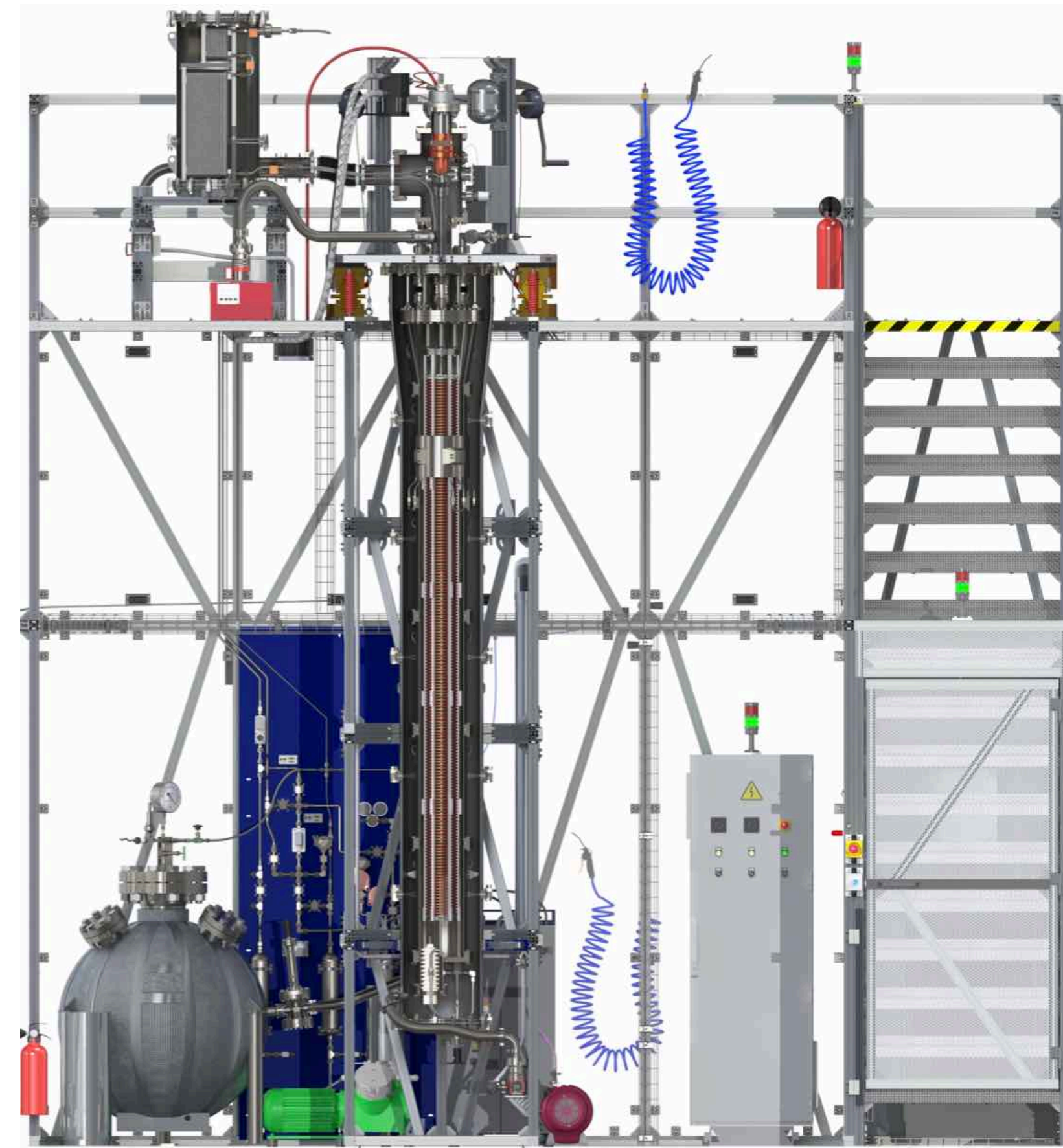
Test e^- drift over 2.6 m (purification, high-voltage): U. Zurich (G-floor Assembly Hall)
