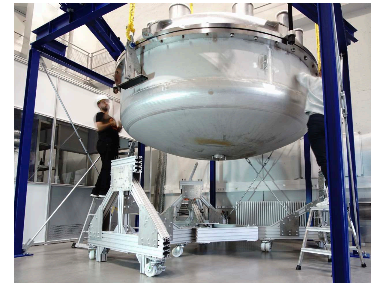
Test electrodes with 2.6 m diameter: U. Freiburg
