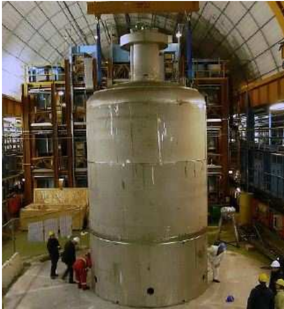
Figure 3.1: The GERDA stainless steel cryostat shortly after its arrival at LNGS in March 2008.
