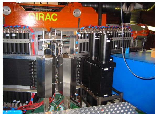
Figure 6.1: Photograph of the three aerogel modules (black) in the experimental area. The scintillation hodoscopes and the N_2 -Čerenkov counter (blue) are also visible.
