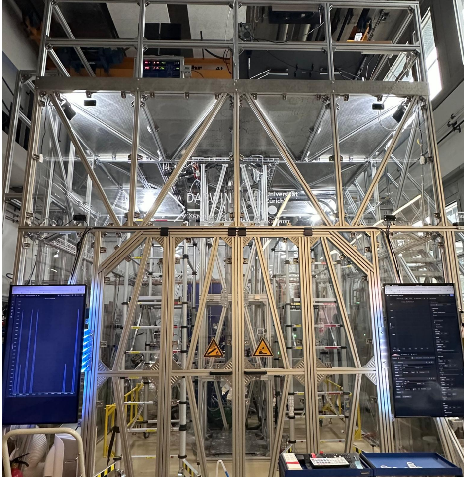
Figure 3: The Xenoscope liquid-xenon research facility at the University of Zurich. The central stainless-steel cryostat houses the liquid-xenon time projection chamber (TPC), while the surrounding aluminium support structure provides mechanical support and access for maintenance. The gas-handling and purification infrastructure is located around and behind the cryostat, and the detector is operated and monitored via the slow-control system displayed on the monitors. Photograph by author.
