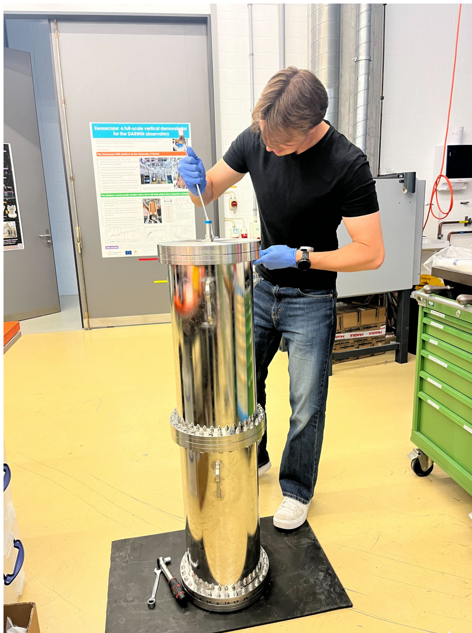
Figure 12: Assembly of the approximately 100 L expansion vessel used to collect the xenon gas after it passed through the HALO moisture analyzer. Photograph by author.
