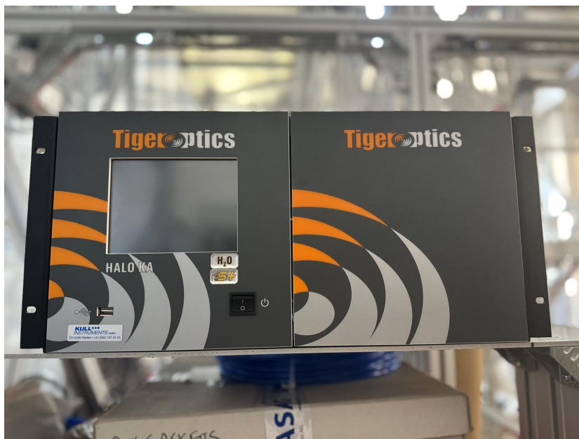
Figure 5: HALO-monitor used in this experiment. Photograph by the author.
