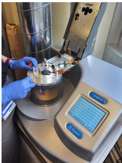
Q150T S automatic sputter coater
