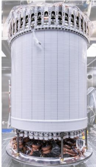
LXe TPC: 7 tonnes of active xenon
