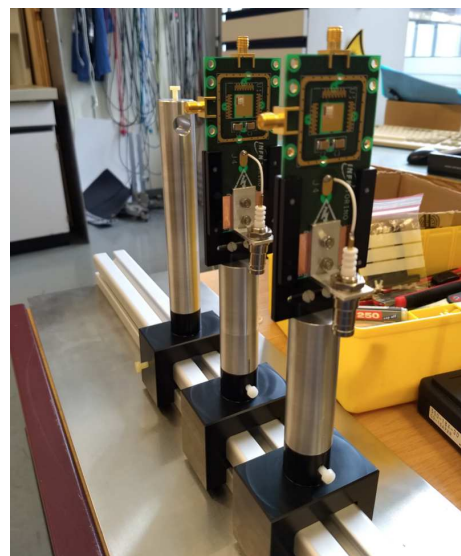
FIG. 9.6 – Part of a setup for testing the timing resolution of LGAD sensors for the Phase-2 CMS pixel detector with a radioactive source.
