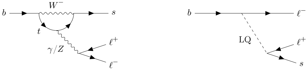
Figure 2.3: Flavor-Changing Neutral Current process b \rightarrow s\ell^+\ell^- in the SM (left) and a NP model involving a scalar leptoquark (right) [9]. In the SM, this necessitates a suppressed loop diagram, while the leptoquark would enable such a decay at tree-level.
