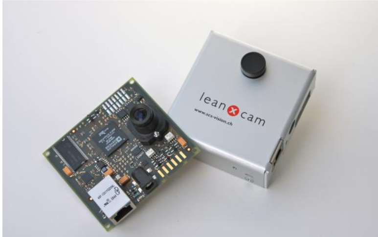
Figure 5.3.: leanXcam case with the camera pcb [33].
