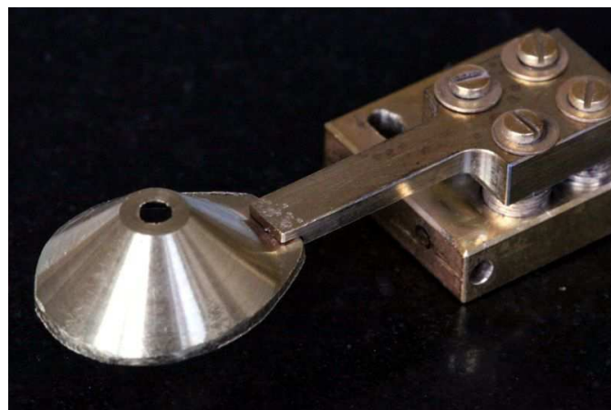
FIG. 16.2 – Dedicated sample holder to guarantee almost zero-field conditions between sample and detector. The opening angle of the cone provides a qualitative impression of the very large aperture of this microscope.
