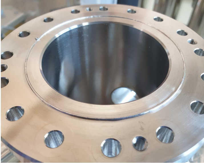
Figure 3.15: Indium seal of the cooling chamber. The indium wire is pressed into a square shaped groove. As seen in the top-left corner, the ends of the wire are twisted and cut to close the ring. The copper cold head sits directly on top of the cooling chamber.
