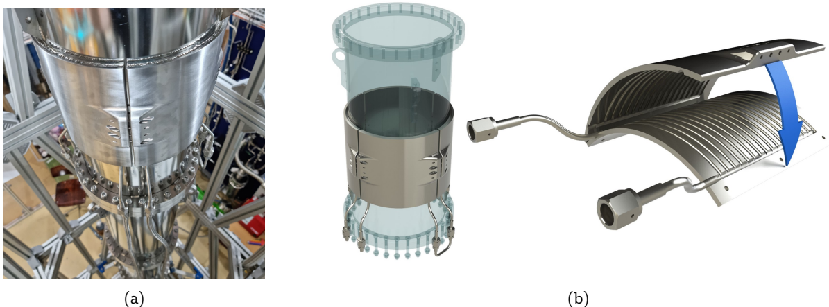
Figure 3.19: Pre-cooler assembly. (a) Pre-cooler installed at the top of the inner vessel. (b) Four pre-cooler plates attached and pressed against the side of an inner vessel section (pale blue). Inside view of a pre-cooling plate. Channels are machined inside the stainless-steel plates to distribute the LN 2 homogeneously. Adapted from ref. [1].
