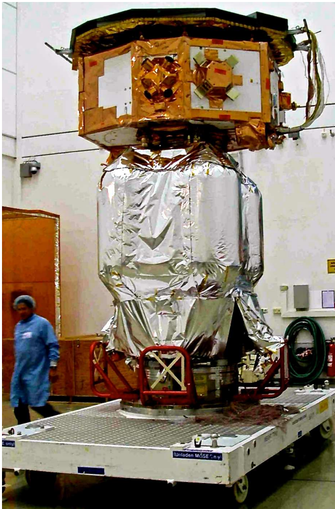
FIG. 2.1 – LISA-Pathfinder at the top of the propulsion module which will bring it at the L1 point (first Sun-Earth Lagrange point).
