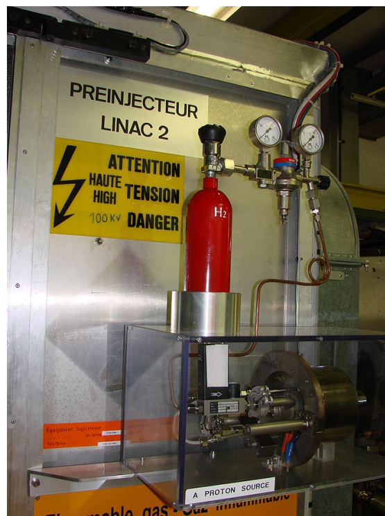
FIGURE 2.2: Hydrogen bottle used to feed protons to Linac2 accelerator. Where it all starts [3]. (Go back to Large Hadron Collider )
